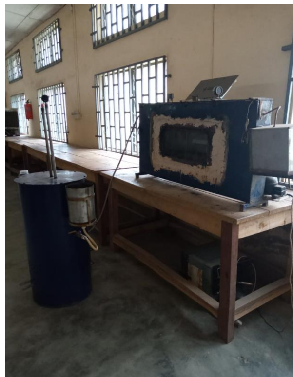
Plate 2: Steam Boiler, SandBox, and Condenser Set-Up
